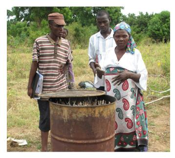
gone an annual internal audit and training with WLRC. The carbonised material is then transported to the WLRC conservancy site and is further processed to produce the final charcoal briquettes or MakaaZingira (In Swahili Zingira means environment and Makaa means charcoal). This is done by adding a mixture of cassava and coir to the carbonised material and by putting this mixture through a briquetting press.
